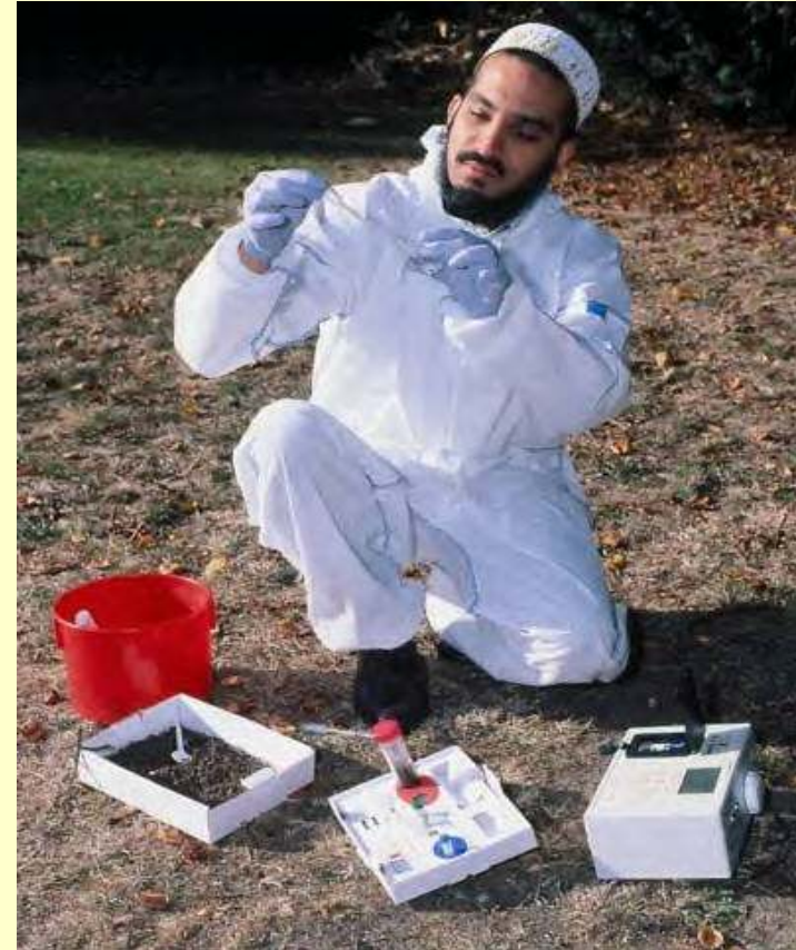
Dr Muffadal Ezzi, senior research scientist tests soil for pollution using the innovative Safe Soil Tester™ (United Kingdom)
